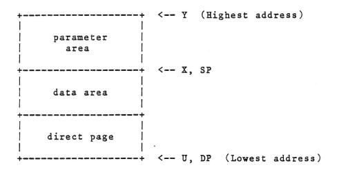
When the process is executed by OS-9, the MPU registers will contain the bounds of the data area: U will contain the beginning address, and Y will contain the ending address. The SP register is set to the ending address+1, unless parameters are used. The direct page register will be set to the page number of the beginning page. If there are no parameters, Y, X, and SP will be the same. Shell will always pass at least an end of line character in the parameter area.
